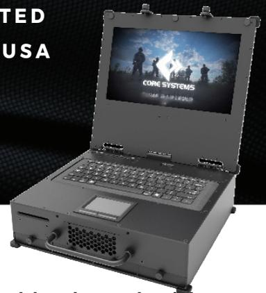
The RPS211D comes equipped with a 11.6" full HD display, sealed keyboard with touchpad and CAC reader. This rugged laptop is engineered for high shock/vibration and temperature. The integrated Intel Xeon 16-Core processor provides true server-class performance while utilizing the onboard PCIe RAID card for high security storage intensive applications.
