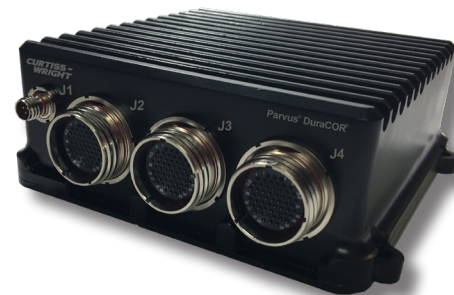
Figure 9: USFF mission computers like the DuraCOR 313 provide small size with modular CPU and I/O architecture
