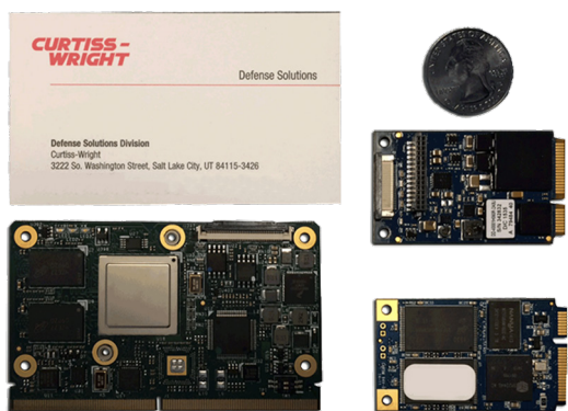
Figure 10: Smaller than a business card processor COM and Mini-PCIe modules
