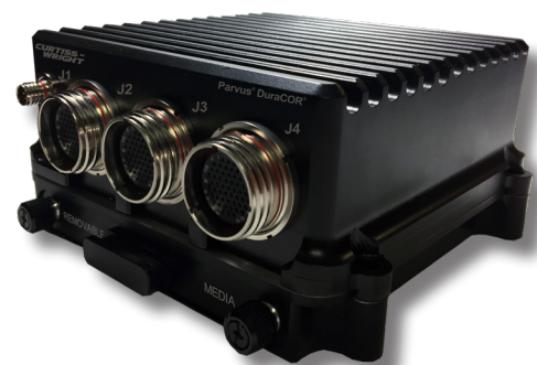
Figure 13: USFF mission computers like the DuraCOR 312 provide small size with modular CPU and I/O architecture
