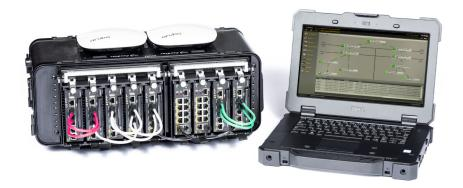
PacStar Secure Wireless Command Post (SWCP) (Wi-Fi) is a small modular communications package enabling wireless mobility for smart phones, tablets, and laptops connected to classified networks (e.g. SIPRnet, MPE, etc.) in deployed, expeditionary, and tactical environments
