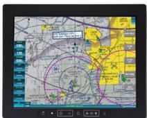
The [PVDU](#) is a 17.3" rugged high definition display with a built-in Intel processor to provide the combined functionality of a mission display and video distribution unit. This has proven to be extremely effective in smaller helicopter platforms to significantly reduce weight and volume. Other display sizes are also available from 10-21".
