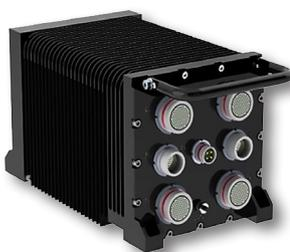
The [MPMC-9321](#) provides all of the key features required for sensor processing including high performance processing, flexible data ingest options, removable storage options and expansion sites to accommodate I/O needs. Processing is achieved using our 3U VPX™ Intel® Xeon® D card at the heart of the system.
